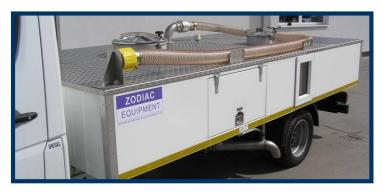
The top wall with manholes with selectable diameter for tank's cleaning and inspecting is covered with aluminium with slip-resistant treatment. 5m waste hose with 4<sup>e</sup> coupler
