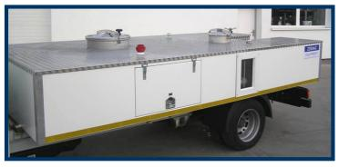
The top wall with manholes with selectable diameter for tank's cleaning and inspecting is covered with aluminium sheet with slip-resistant treatment.
