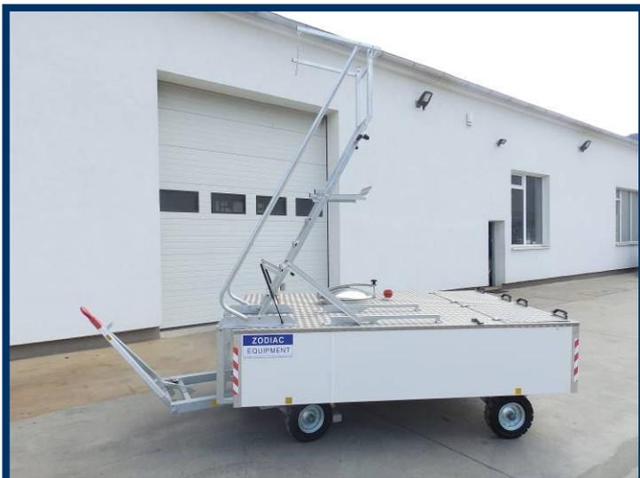
Fixed rear axle forms part of structure. Front axle is steerable on turntable.
