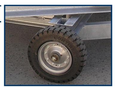
Front axle with turntable steering, rear axle is fixed.
