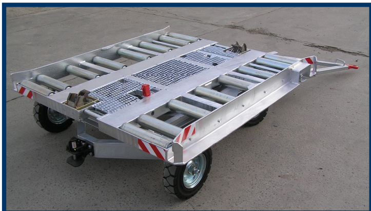
... foldable by pedals located on opposite side of platform.
