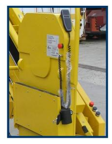
Platform movement can be stopped anytime by stop movement button. Another way to stop device movement is to press any of emergency stop buttons.
