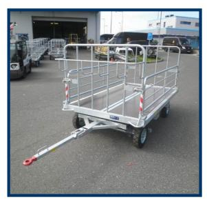
Manual self-locking E-type spring-loaded tow-hitch. Automatic tow-hitch available.
