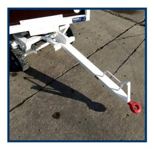
Manual self-locking E-type spring-loaded tow-hitch. Rockinger tow-hitch available.
