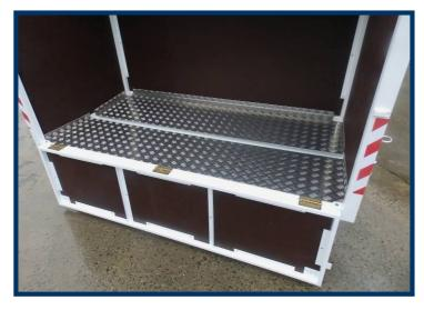
Loading platform made out of two V shaped aluminium anti-skid sheets,
