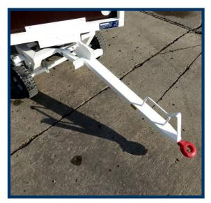
Manual self-locking E-type spring-loaded tow-hitch.
