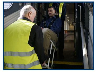
The airchair is designed for easy manipulation in limited space inside of aircrafts.
