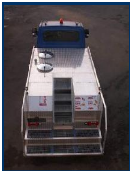
The top wall is covered with an aluminium sheet with slip-resistant treatment.
