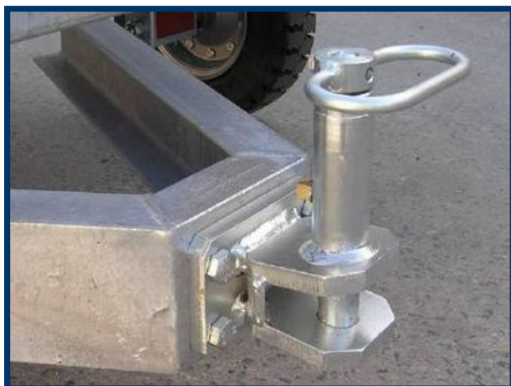
E-type manual spring-loaded tow hitch.
