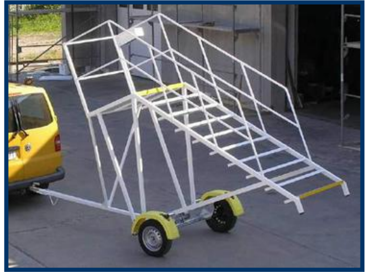
1 fixed axle with standard car trailers wheels.
