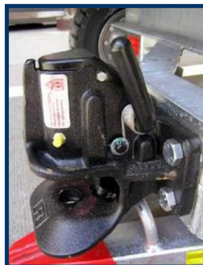
E-type manual spring-loaded tow hitch.
