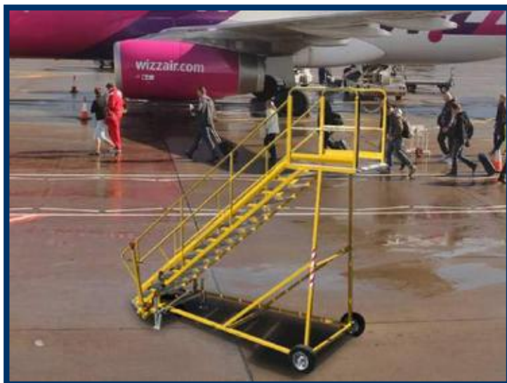
4 wheels with steel discs, ball bearing hubs and solid rubber tyres.
