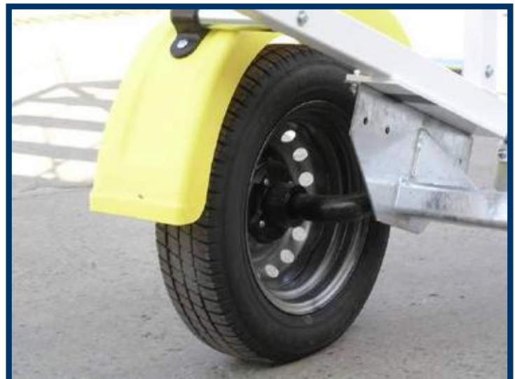
1 fixed axle with standard car trailers wheels.
