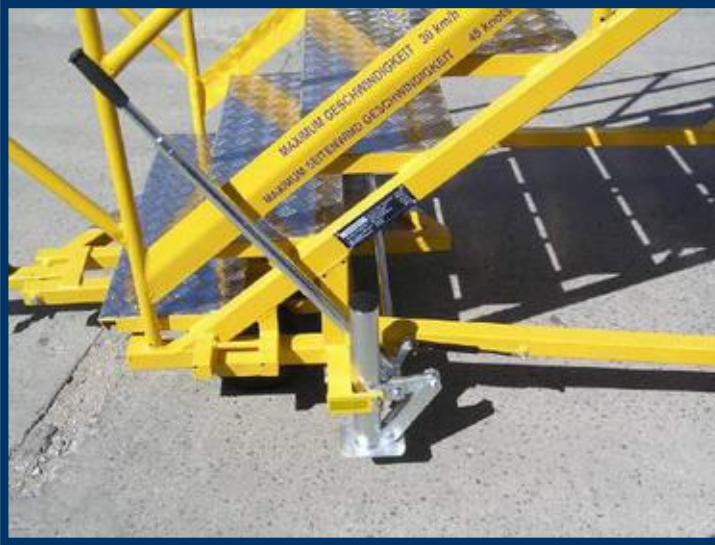
Stability in the operational position is provided by two manually operated stabilizers.
