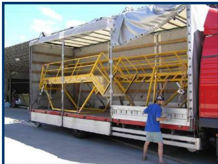
Since the construction allows removal of the front axle frame, 2 pieces can be transported by 1 truck with about 7m of cargo space length.
