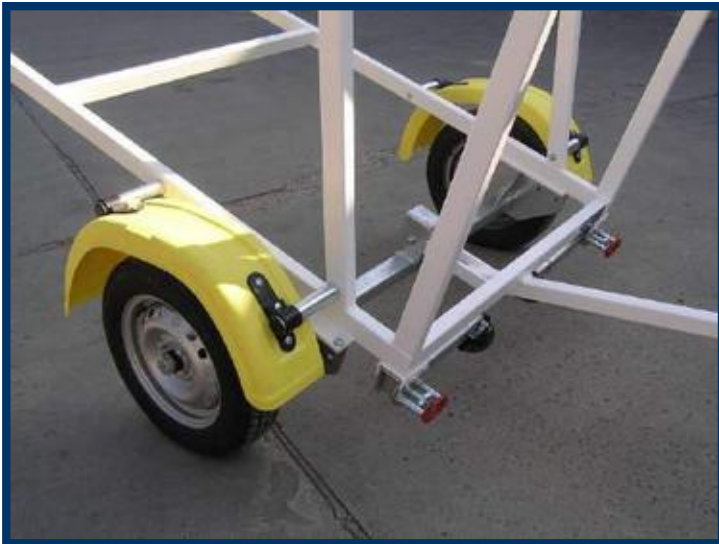
1 fixed axle with standard car trailers wheels.
