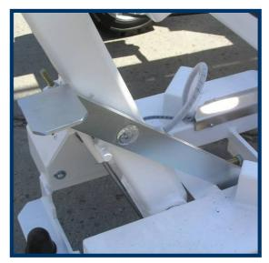
Front part of upper platform flexibly retractable 100 mm, equipped with protective bumper.
