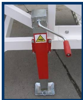
4 jacks for height adjustment.
